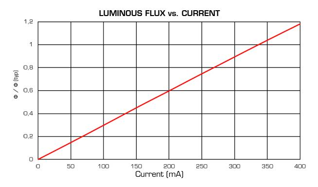
Due to the special conditions in the production process of LEDs, the specified values are statistical averages. The individual LED may deviate from them.
