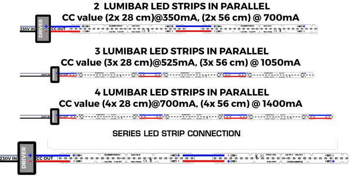
The series connection is applied by connecting the positive (+) terminal of the first LED strip to the negative (-) terminal of the second LED strip. This pattern is repeated for further LED strips, from the negative (-) of the second strip to the positive (+) of the third strip and so on. At the same time, the negative (-) of the first LED strip is wired to the (+) of the second, then the (-) of the second to the (+) of the third and so on.
