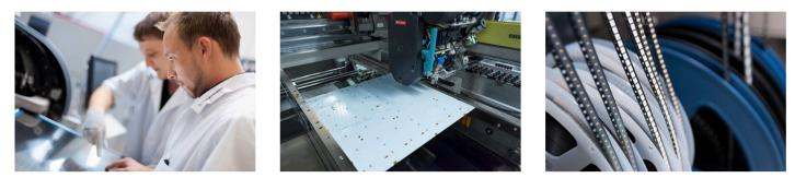
The LumiBar is **made in Germany**, at a production line that uses the innovative manufacturing technology of plasma direct metallization, to turn substrates into electrical conductive and solderable circuit boards, even those that before have not been suitable for an assembly with electronic components.
