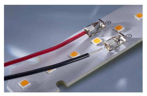
The professional LED strip is connected via a solderless connection to the connection inputs provided for this purpose.
