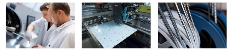
This LED strip is **made in Germany**, at a flex production line that uses the innovative manufacturing technology of plasma direct metallization, to turn flexible substrates into electrical conductive and solderable circuit boards, even those that before have not been suitable for an assembly with electronic components.
