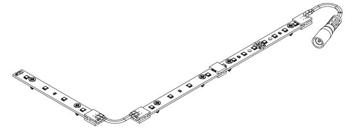
The Multibar easy to use plug-fit system allows the strips to be connected into long light strips with evenly spaced LEDs. No soldering is required.
