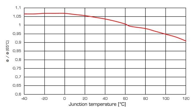
LUMINOUS FLUX vs. TEMPERATURE
