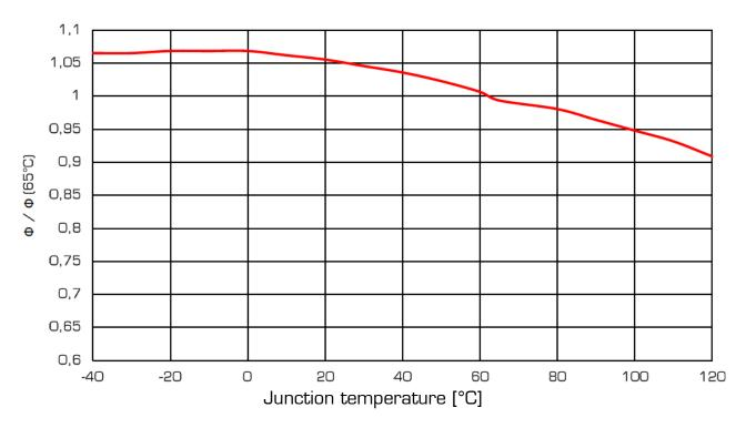
LUMINOUS FLUX vs. TEMPERATURE
