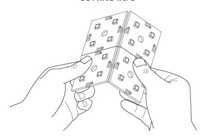
The LED module can be separated into smaller units up to 1 single module of 30x30mm. The connectors work on the separated parts also.
