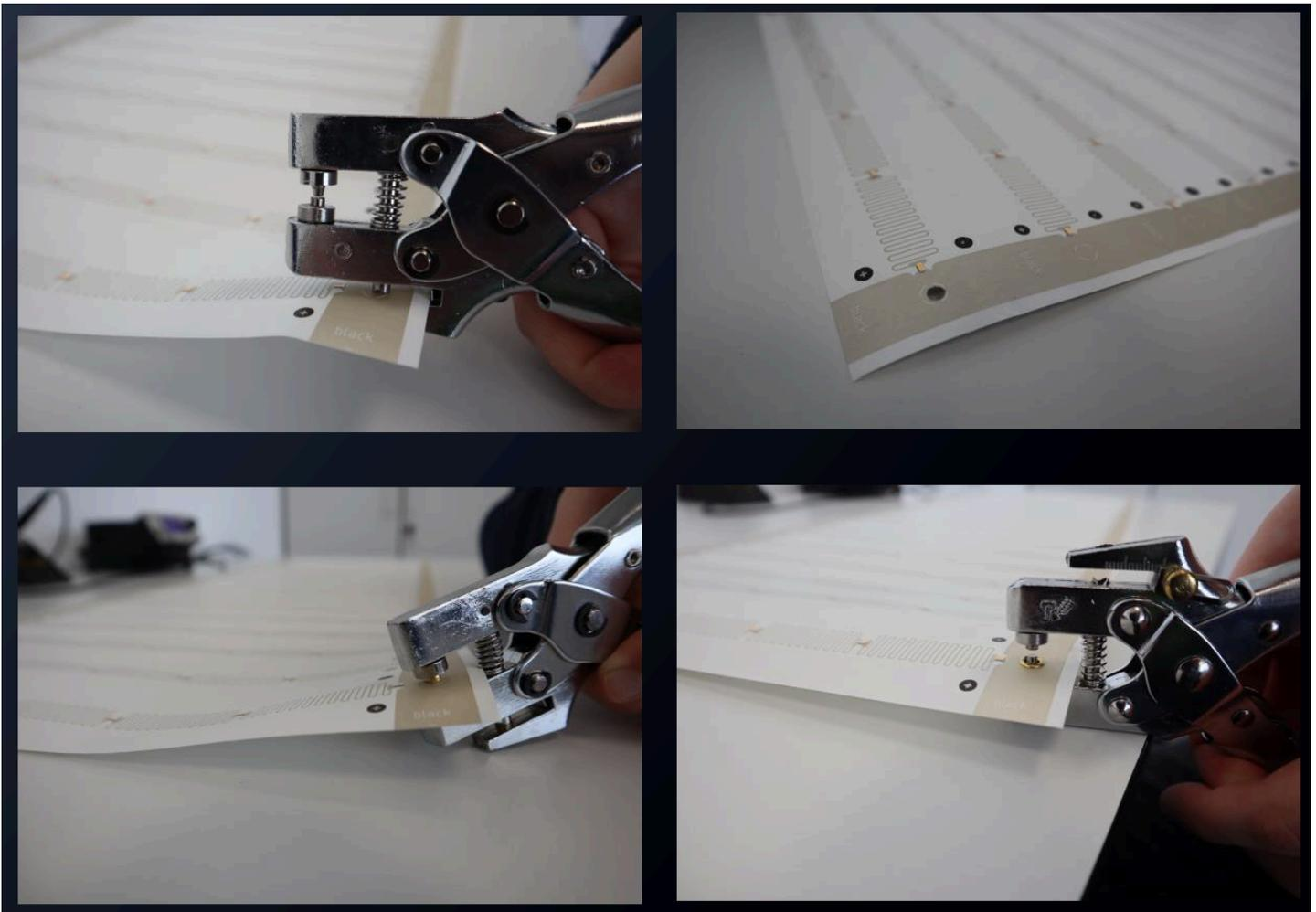
The PaperFlex1080 can be connected to wires via a Eyelet Pliers tool, such as found here:
