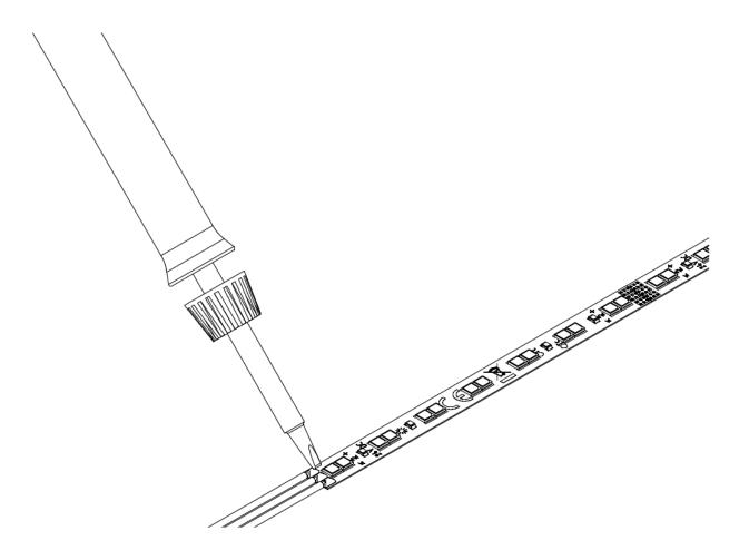
The Professional LED Strips are connected via a lead connection to the connection pads provided for this purpose.
