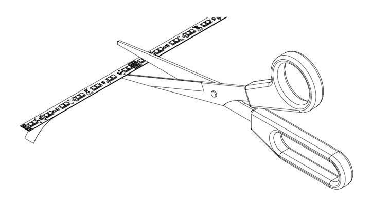
The LED strip can be separated or shortened every 100 mm. On the back of the LED strip is a double-sided heat-conducting adhesive tape, which allows installation of the LED strip. Professional LED strips can be cut with scissors.
