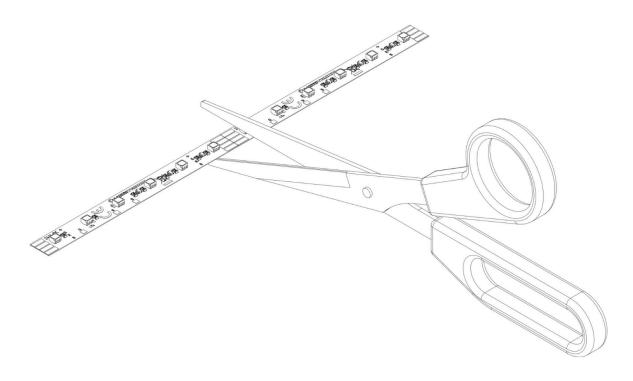
The LED strip can be separated or shortened every 100 mm. On the back of the LED strip is a double-sided heat-conducting adhesive tape, which allows installation of the LED strip. Professional LED strips can be cut with scissors.
