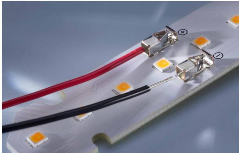
The professional LumiBar strip is connected via a solderless connection to the connection inputs provided for this purpose. **The form factor and connection is designed according to the Zhaga standard (Book 7 L28W2).** The wire insulation has to be removed at the connection point. Recommend wire cross-section of inner conductor:  $2 \times 0.75 \text{ mm}^2$  (AWG 18).
