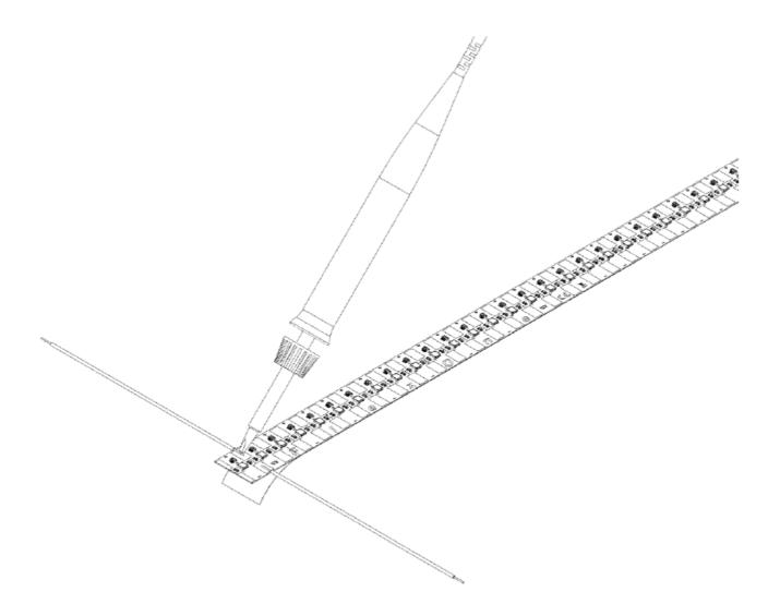
The Professional LED Strips are connected via a lead connection to the connection pads provided for this purpose.
