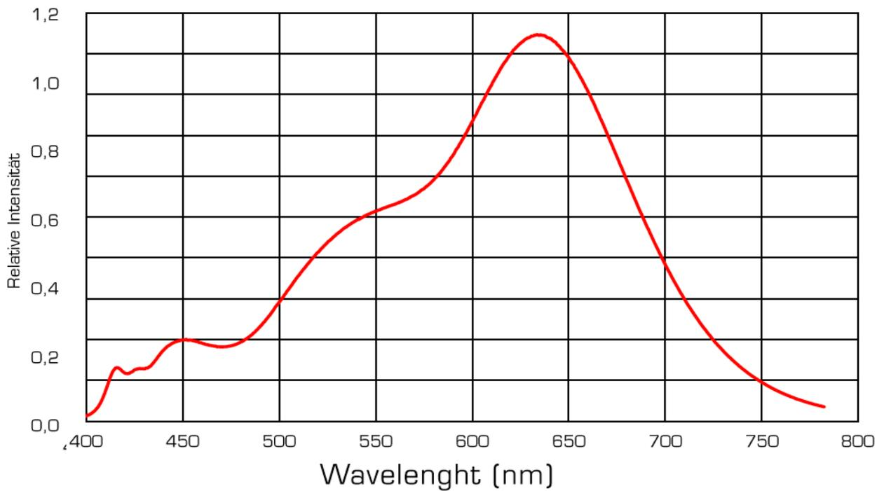
LUMIFLEX3098+ TOSHIBA-SSC LED STRIP SUNLIKE CRI98 WARM WHITE 2700K 8450LM 24V 140 LEDS/M 5M REEL
