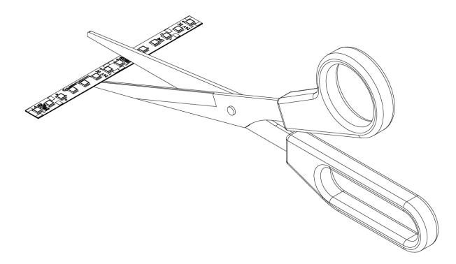
The LED strip can be separated or shortened every 50 mm. On the back of the LED strip is a double-sided heat-conducting adhesive tape, which allows installation of the LED strip. Professional LED strips can be cut with scissors.
