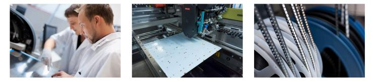
This LED strip is **made in Germany**, at a flex production line that uses the innovative manufacturing technology of plasma direct metallization, to turn flexible substrates into electrical conductive and solderable circuit boards, even those that before have not been suitable for an assembly with electronic components.
