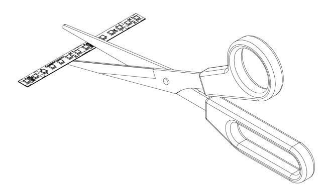
The LED strip can be separated or shortened every 280 mm which is equal to the length of a single module of 900mA at 8.25V. On the back of the LED strip is a double-sided heat-conducting adhesive tape, which allows installation of the LED strip. Professional LED strips can be cut with scissors.
