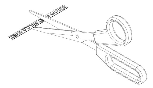
The LED strip can be separated or shortened every 280 mm which is equal to the length of a single module of 900mA at 8.25V. On the back of the LED strip is a double-sided heat-conducting adhesive tape, which allows installation of the LED strip. Professional LED strips can be cut with scissors.
